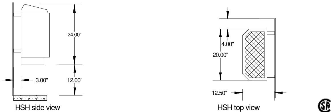
Figure 2. HSH clearances to wood surfaces
